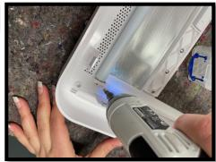
Locate the end of the blind with the metal pin and remove the 3 screws which hold the plastic retaining strip. 2
