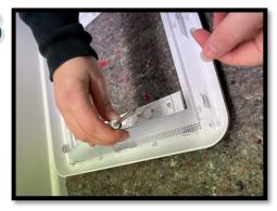
CAUTION! The roller blind is spring loaded. Carefully remove the metal end of the blind from its recess.
