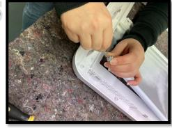
Carefully place the end of the blind back into the recess. Be careful not to release the blind as this will cause the tension to slide.
