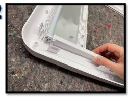
Remove the plastic retaining strip.
