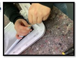
Holding the blind in place, wind the metal bar clockwise until tension builds up (approx. 4-5 turns).
